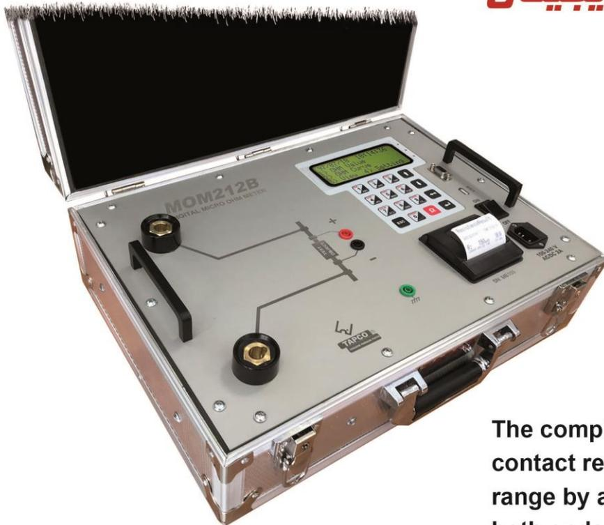
The complete toolbox for measuring contact resistance in the micro ohm range by applying high current to both ends.
